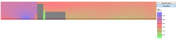
b) Cross-sectional simulation results for the eastern boundary (with solid walls and multi-story buildings parallel to the street)
