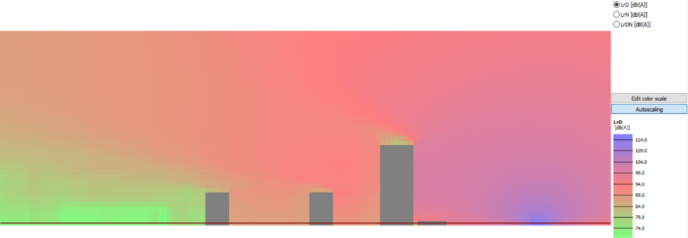
c) Cross-sectional simulation results for the southern boundary (Right 1: High-rise building is Teaching Building 3; Right 2: Student Dormitory 7; Left 1: Student Dormitory 6; no solid wall)
