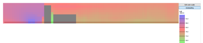
b) Cross-sectional simulation results for the eastern boundary (with solid walls and multi-story buildings parallel to the street)
